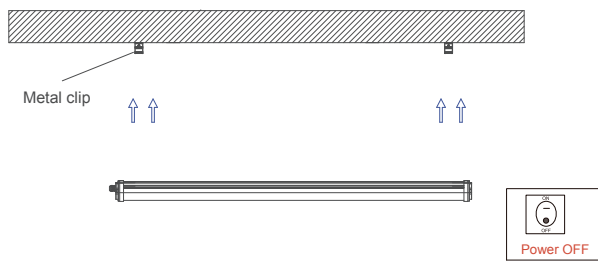
C: Install the lamp into the clips.
